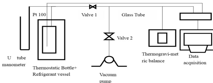
**Figure 3 :** *Experimental setup of the thermogravimetric balance system*
