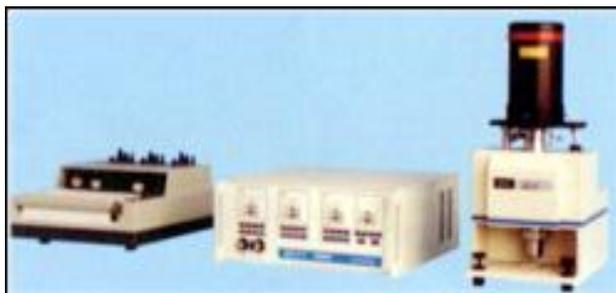
**Figure 2 :** *Photograph of thermobalance and accessories*
