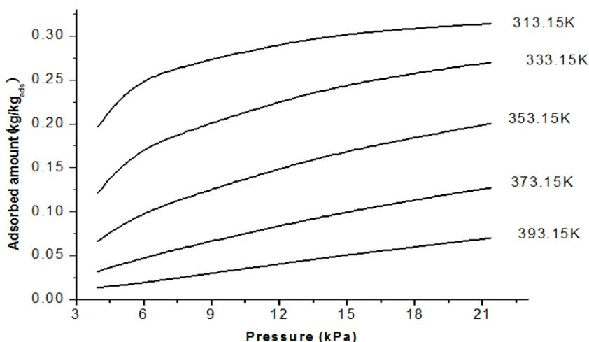
**Figure 4 :** Calculated adsorption capacity vs. pressure of methanol- AC
