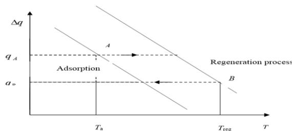
**Figure 1** : Adsorption - regeneration cycle shown in isobaric diagram
