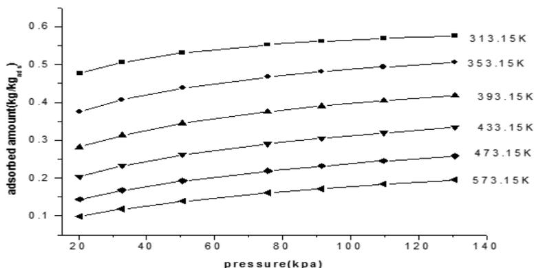
**Figure 5 :** Calculated adsorption capacity vs. pressure of R123-AC
